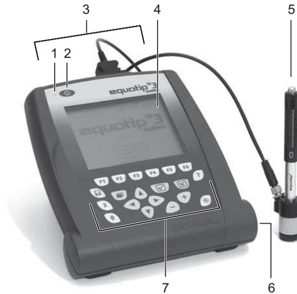
Fig. 2.01 Electronic indicating device
