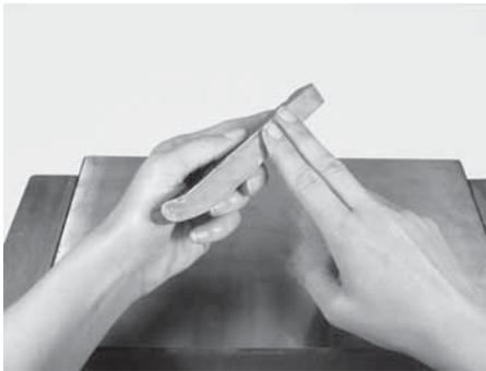
Fig. 6.01 Application of coupling paste
