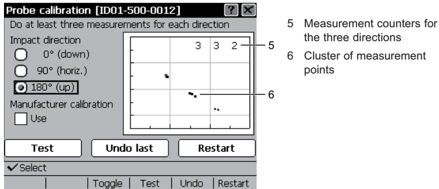
Fig. 4.06 Probe calibration
