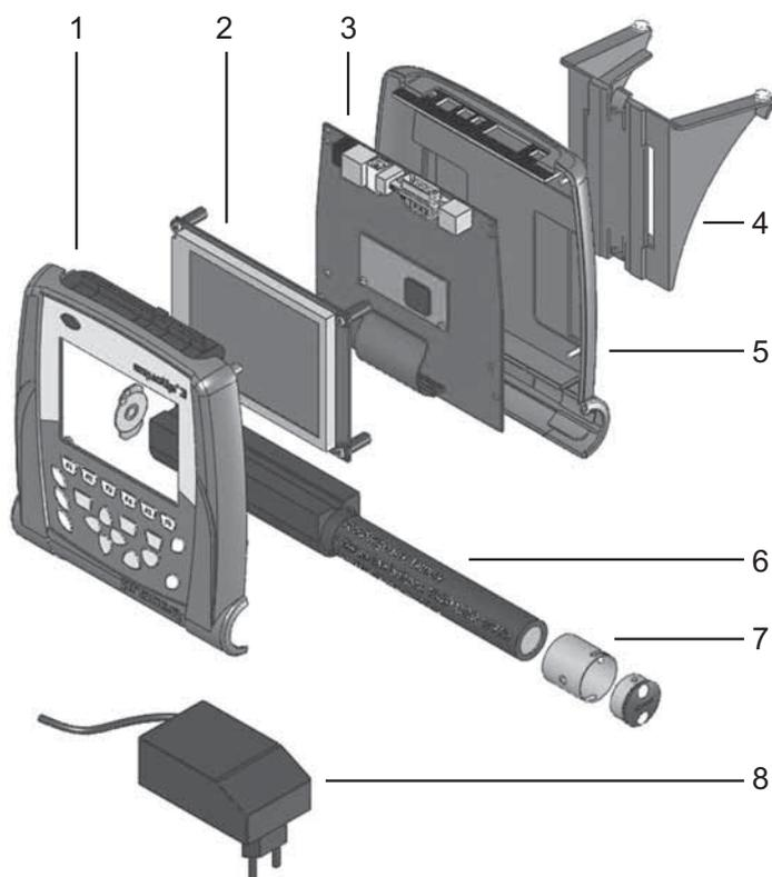
Fig. 9.01 Explosion drawing EQUOTIP® 3 indicating device
